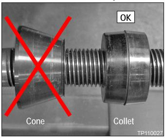
Determine the road wheel-to-collet contact area for proper centering (see below).
