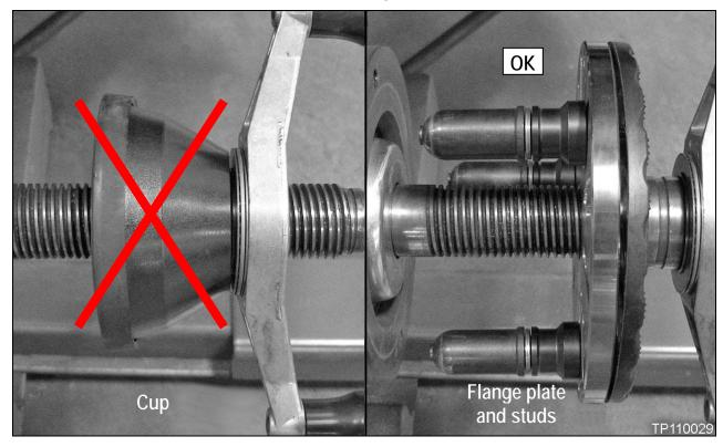
Properly mount the tire/wheel assembly to the wheel balancer (see below).
