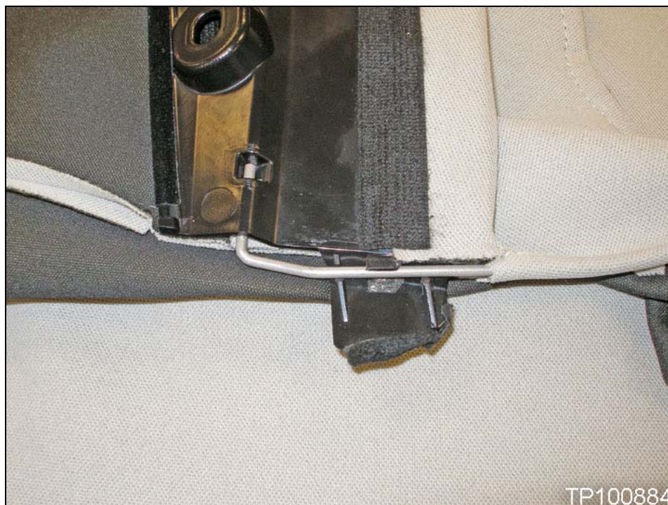
Wire rod properly installed
