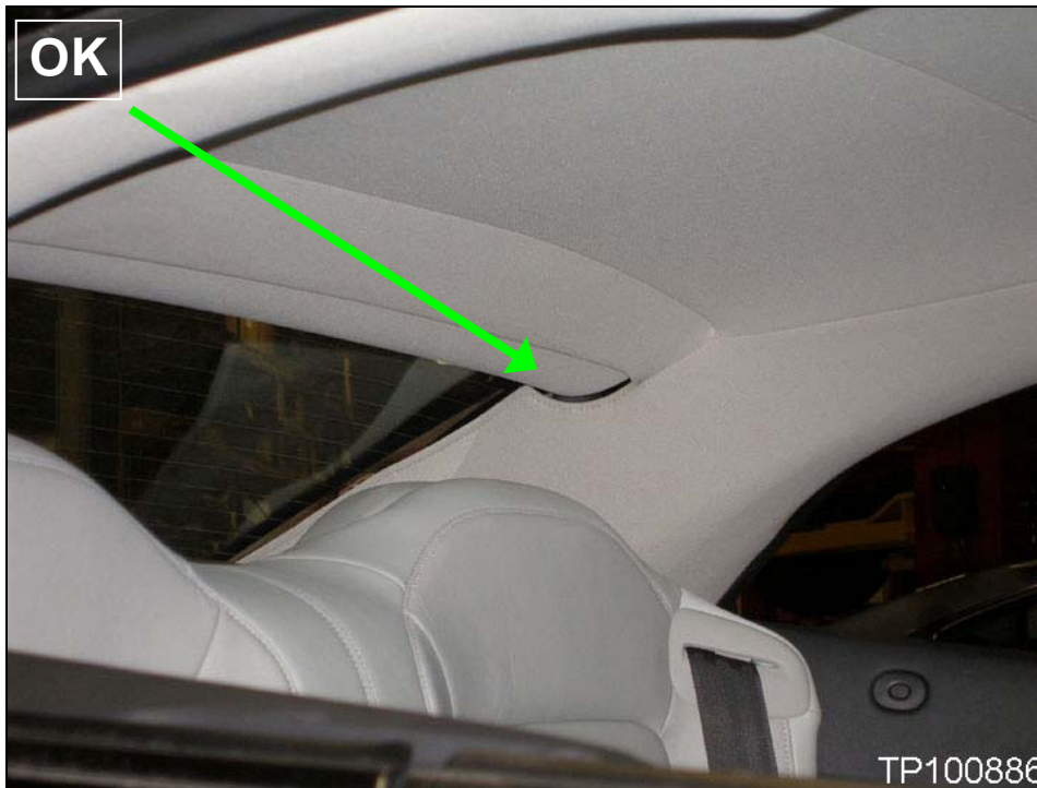
Wire rod properly installed
